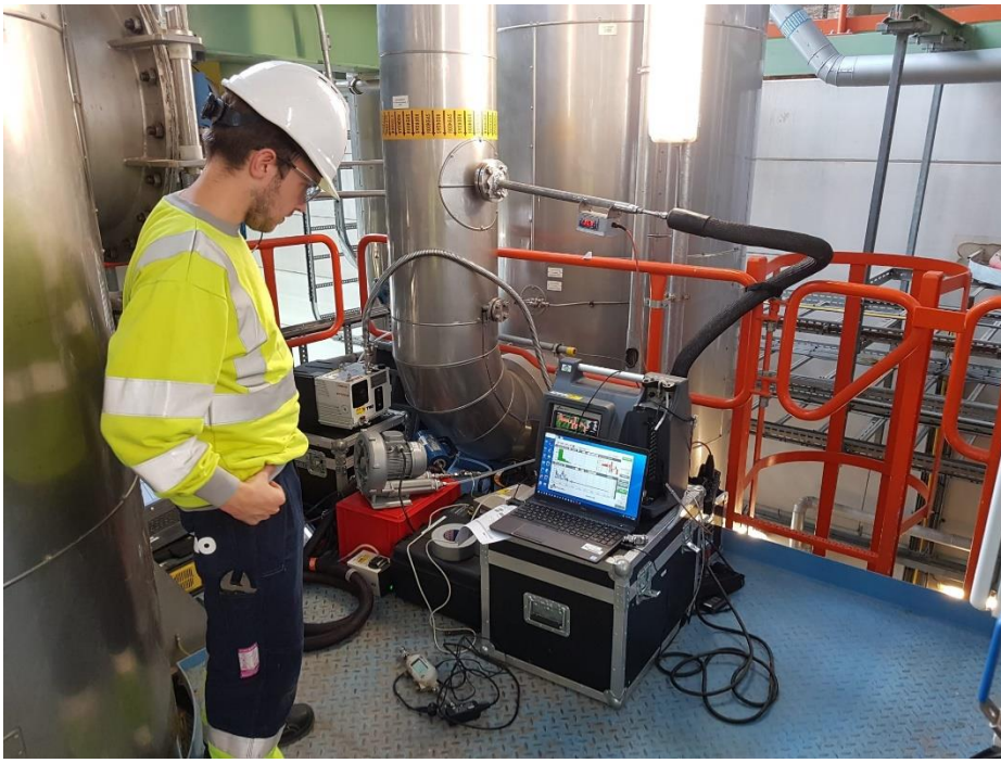
Figure 1. ELPI connected to a flue gas line at Twence's CO 2 capture pilot plant
