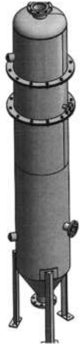
3D acid wash column. The total height of the column is 4.7 m from the base to the top
