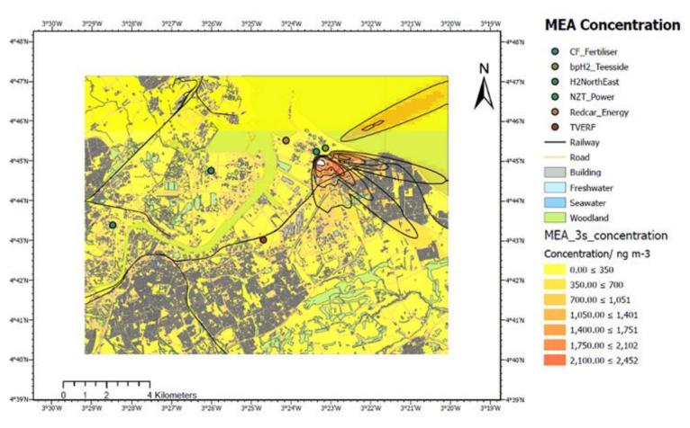
Atmospheric ground-level concentrations varying as a function of distance from emitting PCC facilities UK case study (single facility and multiple facility studies)
